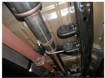
**Step 4.** Loosely install the supplied Hanger Clamp Assembly to either the Inlet Pipe Assembly or the Extension Pipe depending on your vehicles configuration. Locate the welded hanger to the forward rubber insulator as shown.
