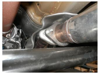
**Step 3.** Begin installation by loosely attaching the Inlet Pipe Assembly to the OEM flange outlet using the supplied hardware.
