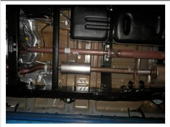
**Step 1.** To remove the OEM exhaust system, loosen the factory clamp forward of the muffler. Loosen the nuts attaching the resonator assembly to the flange junction. Rotate the resonator assembly to release the muffler inlet locking boss. Remove the nuts at the inlet flange. Working front to rear disengage all welded hangers from the rubber insulators and remove the OE system. Be sure to retain all mounting hardware as it will be needed to install your new MagnaFlow system.
