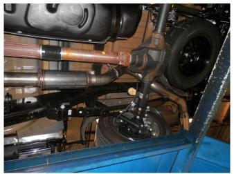
**Step 7.** Loosely install the Tail Pipe Assembly using the supplied clamp. Engage the welded hanger to the rubber insulator.
